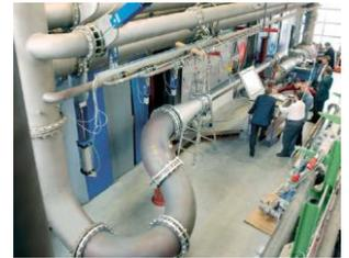
Level 1: If sufficient straight inlet and outlet pipe sections are available, the **VACOMASS® flow meter** receives the system-specific standard calibration as a single meter. The process conditions such as installation situation, pipe orientation, flow range, pressure and temperature are taken into consideration. This ensures a high accuracy of measurement.
