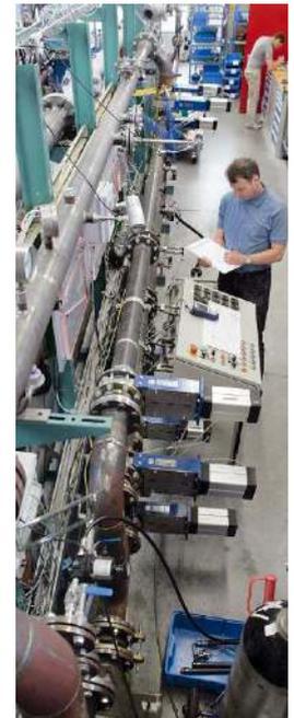
Level 3: If pulsations are to be expected or if the inlet section is far too small, a **VACOMASS® flow conditioner** can be used upstream. The calibration is carried out as a compact unit of flow meter, flow conditioner and possibly the control valve.
