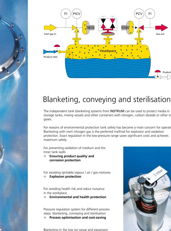
The independent tank blanketing systems from **INSTRUM** can be used to protect media in storage tanks, mixing vessels and other containers with nitrogen, carbon dioxide or other inert
